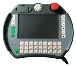
Enmair robot controller is an innovative product, based on the CNC control core, the algorithm includes six joint robot, six joints used in robot control, with series controller adopts the same software interface, reduce the burden of learning, the ways of application of the elastic can be widely used in a variety of purposes, rich communication function, is the best tool for automated integration.
